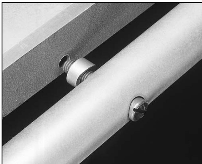
Figure 24. Attaching fence rails.
